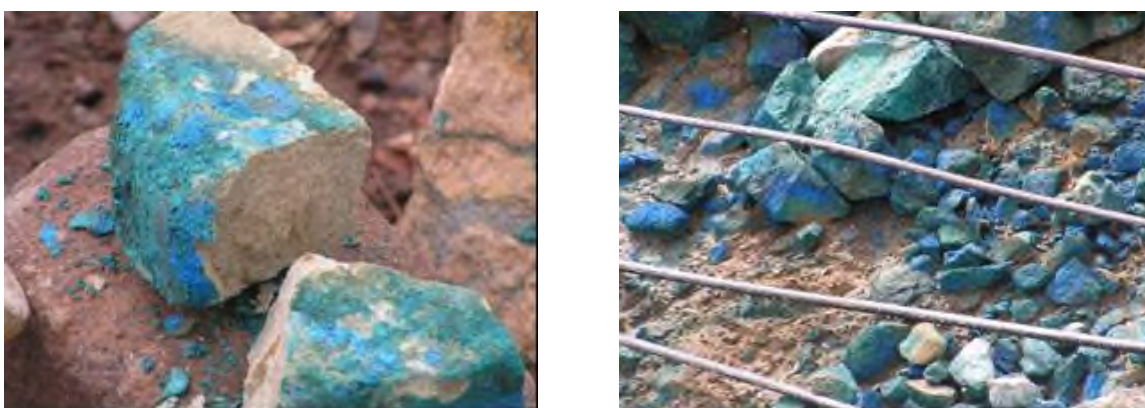
Broken ore particle from the Leon heap leach (left) and overview of the heap (right) after the ore-specific pre-treatment stage
